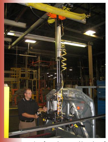
A US car manufacturing plant needed to be able to transfer hood components safely from a conveyor to a storage rack without causing product damage.
